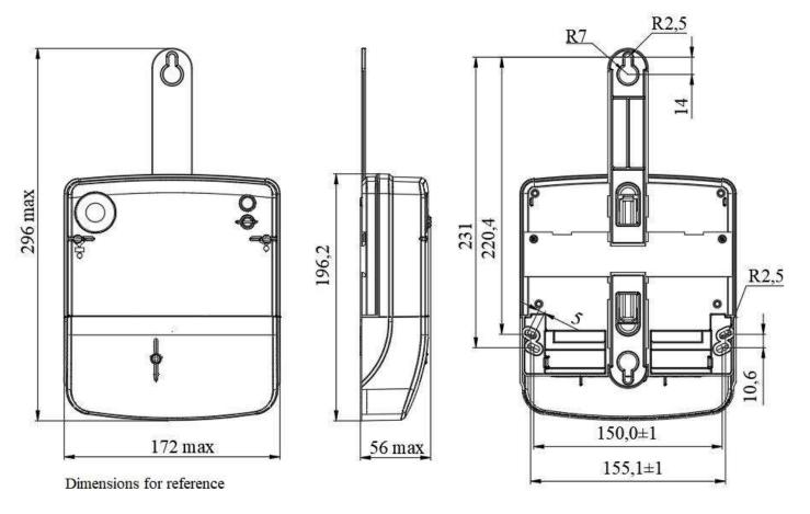
Figure A. 1. Overall and installation dimensions of meters
