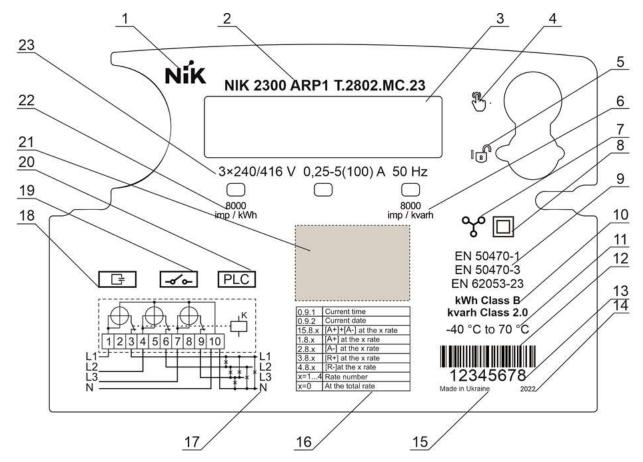
Figure 3. Example of NIK 2300 ... P1... nameplate design
